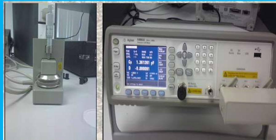
Agilent E4980A precision LCR meter and the 16451B dielectric test fixture
