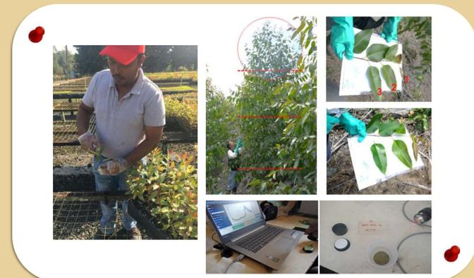
Figure 1. left. Process flow of calibration development and right is foliar sampling at nursery, field stage and sample scanning using a microNIR 1700 (Viavi Solutions, Milpitas, CA, USA)
